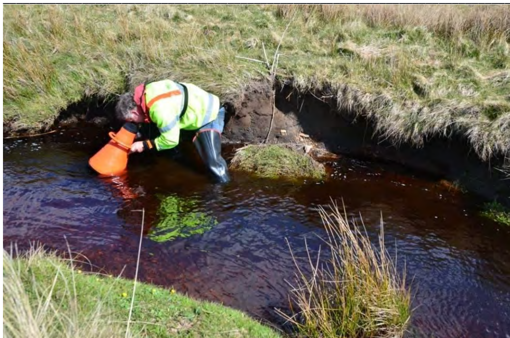
Figure 1 Use of bathyscope to view river bed.
