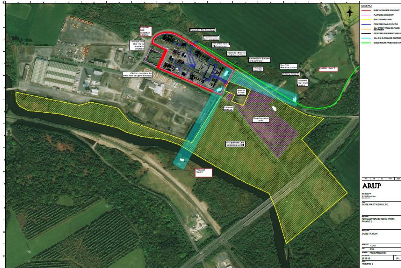
Figure 6: Proposed Substation Site Layout
