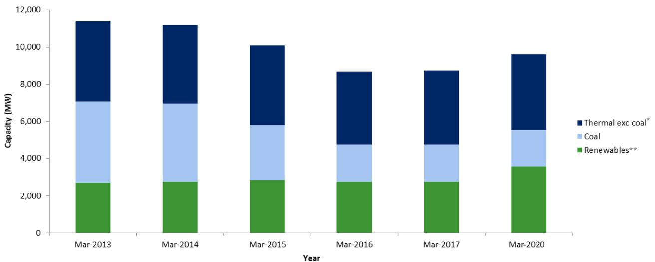
\* Thermal non-coal is mainly gas-fired CCGT's with c.150MW of island diesel generation and up to 70MW of multifuel generation.
