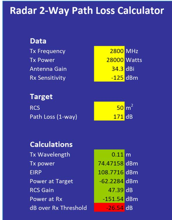
Figure 8: Path loss calculation for turbine C1
