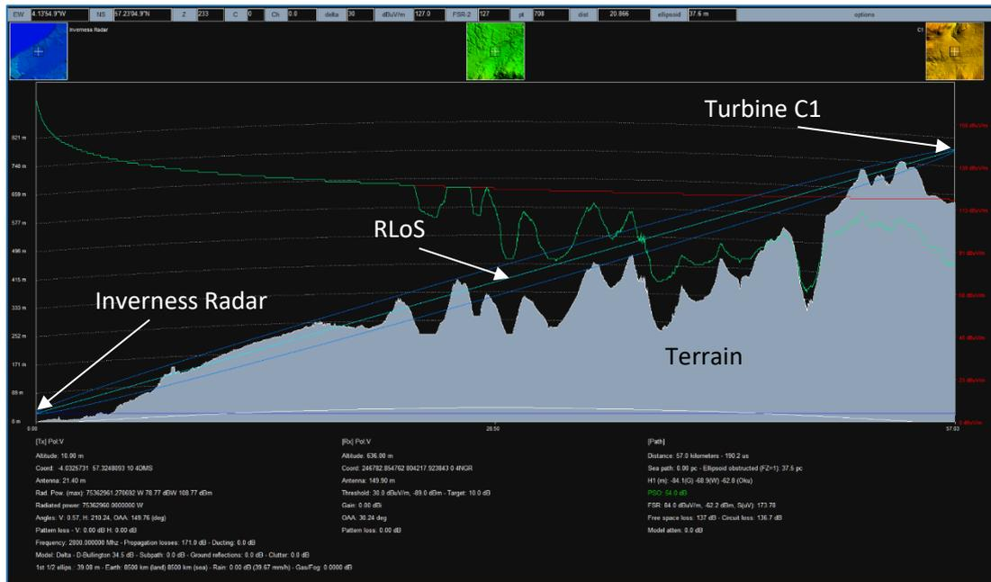
Figure 7: Path profile between Inverness Radar and turbine C1
