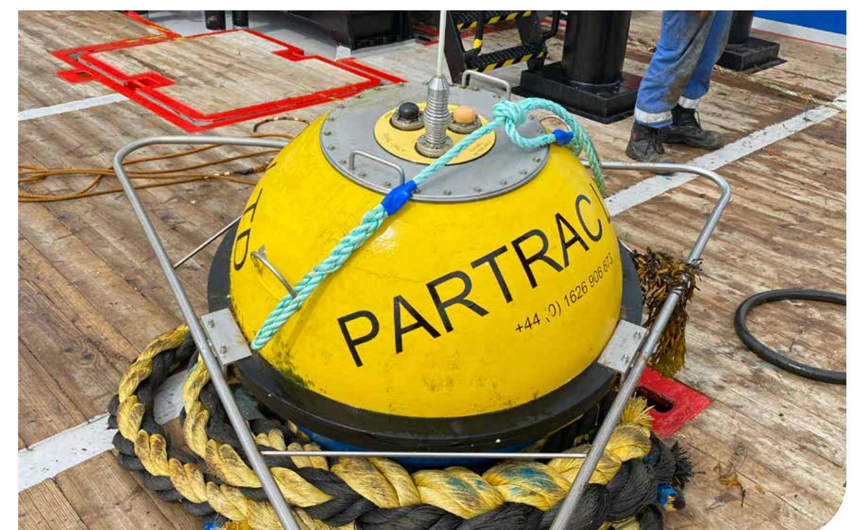
Wave buoy as part of the metocean survey
