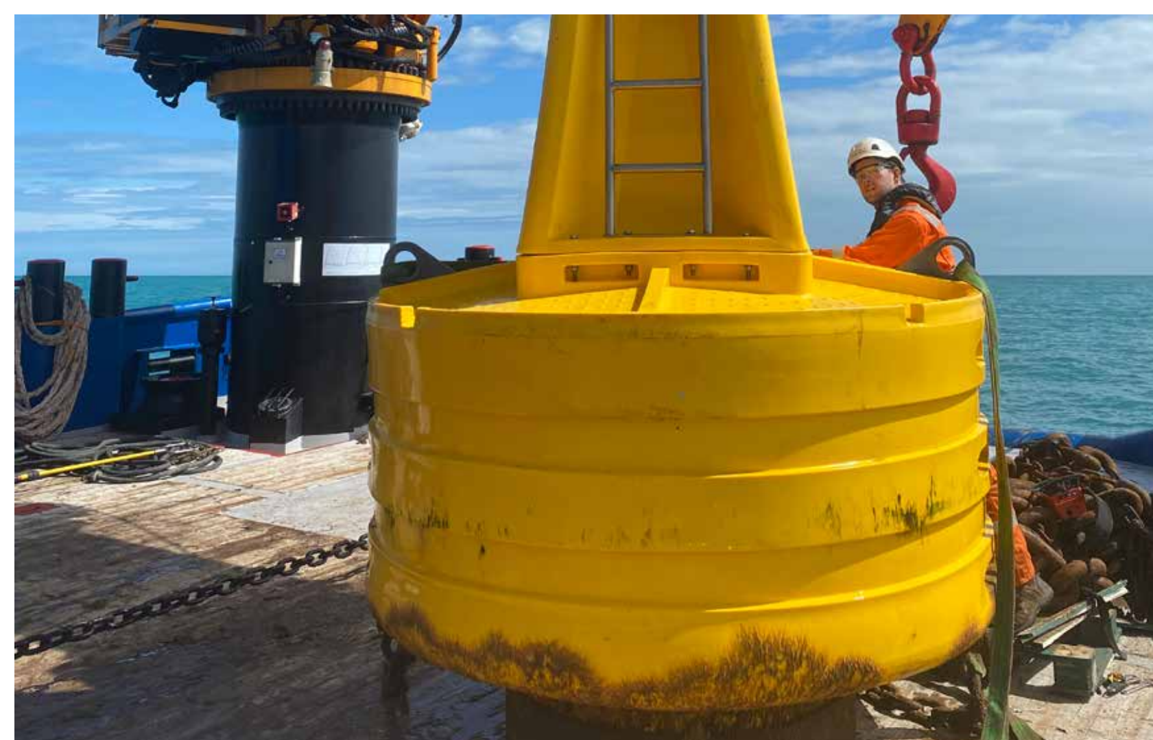
Guard buoy used as a marker as part of the metocean survey
