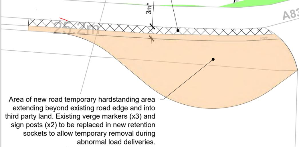
Area of new road temporary hardstanding area extending beyond existing road edge and into third party land. Existing verge markers (x3) and sign posts (x2) to be replaced in new retention sockets to allow temporary removal during abnormal load deliveries.
