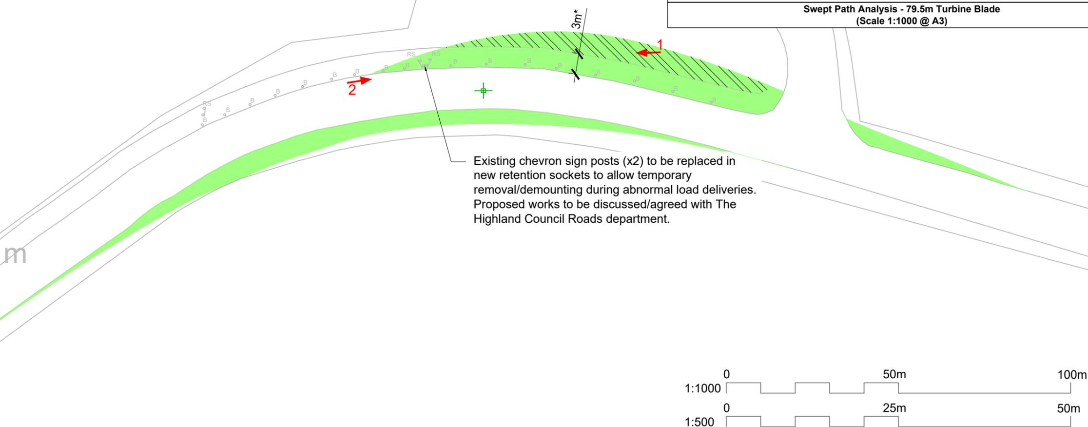
Existing chevron sign posts (x2) to be replaced in new retention sockets to allow temporary removal/demounting during abnormal load deliveries. Proposed works to be discussed/agreed with The Highland Council Roads department.
