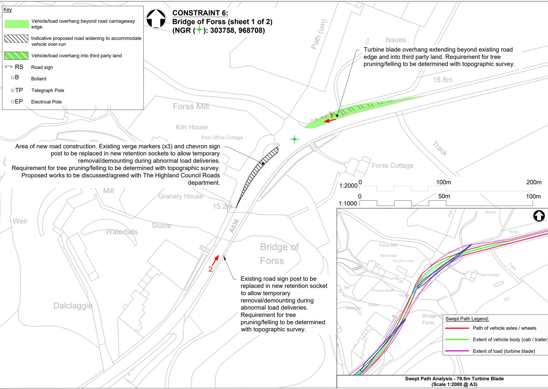
Area of new road construction. Existing verge markers (x3) and chevron sign post to be replaced in new retention sockets to allow temporary removal/demounting during abnormal load deliveries. Requirement for tree pruning/felling to be determined with topographic survey. Proposed works to be discussed/agreed with The Highland Council Roads department.
